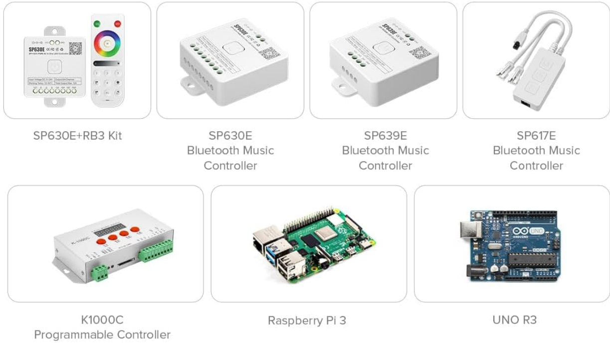
Image 6.1: Examples of compatible controllers for the LED strip, including K1000C, SP630E, SP639E, SP617E, SP530E, Raspberry Pi, and Arduino UNO R3.
