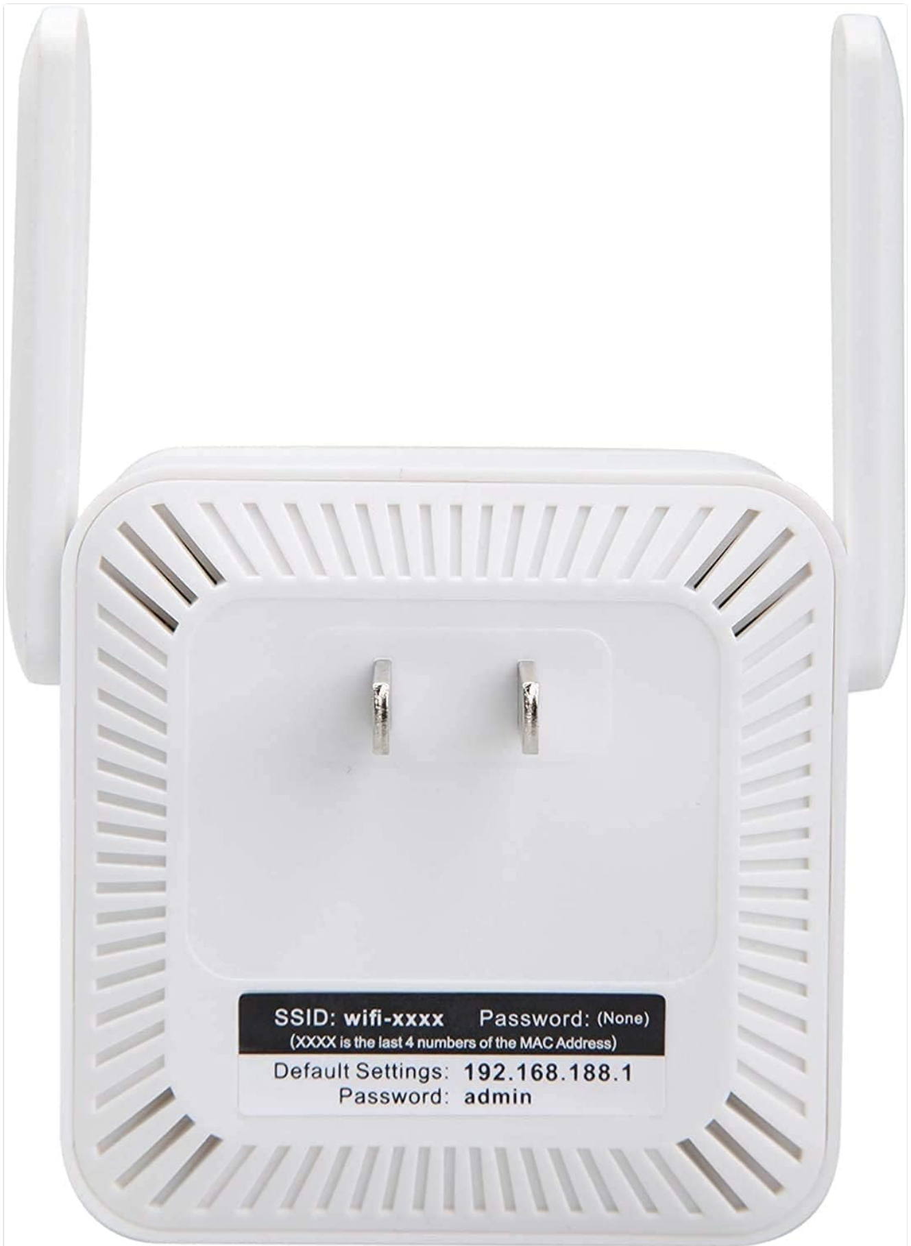
Image: Back view of the Aimery WiFi Extender, displaying the default SSID format (wifi-xxxx) and the default settings IP address (192.168.188.1) and password (admin).
