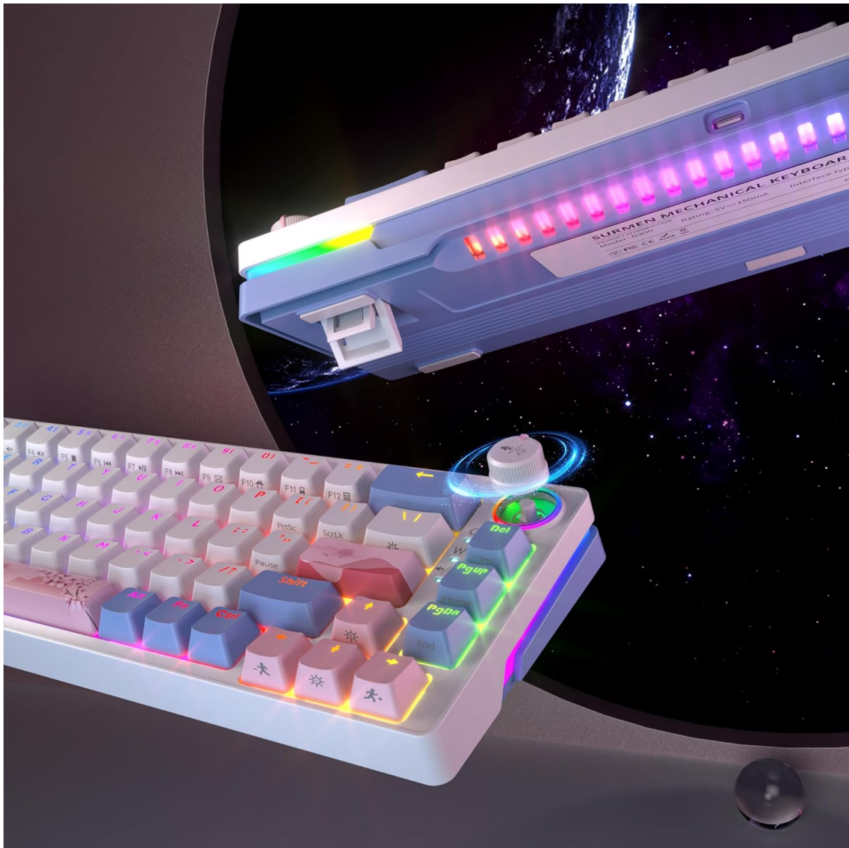
Figure 4: RGB Backlighting and Volume Control Knob
