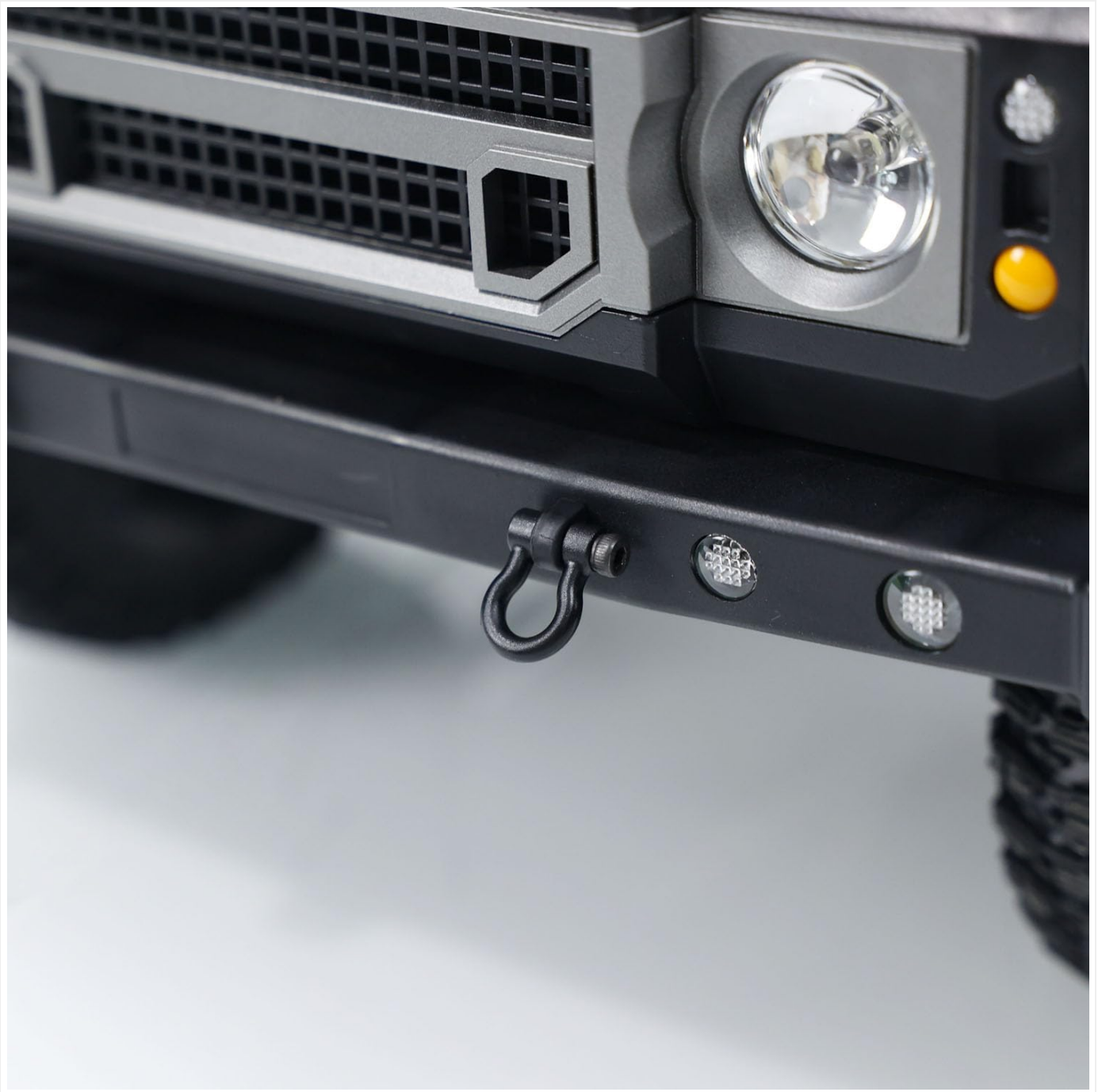
Figure 4: Detail of the front bumper with integrated tow hook, indicating robust design for off-road use.
