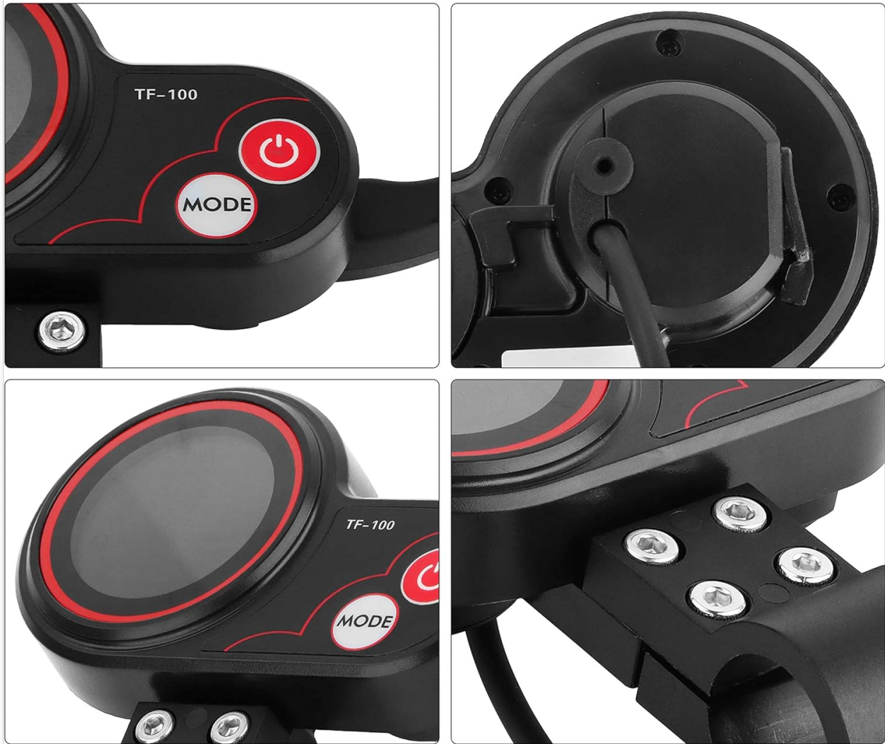
Figure 4.2: Close-up details of the TF-100 unit, showing the display, power button, mode button, and the thumb throttle mechanism. The robust construction is visible.
