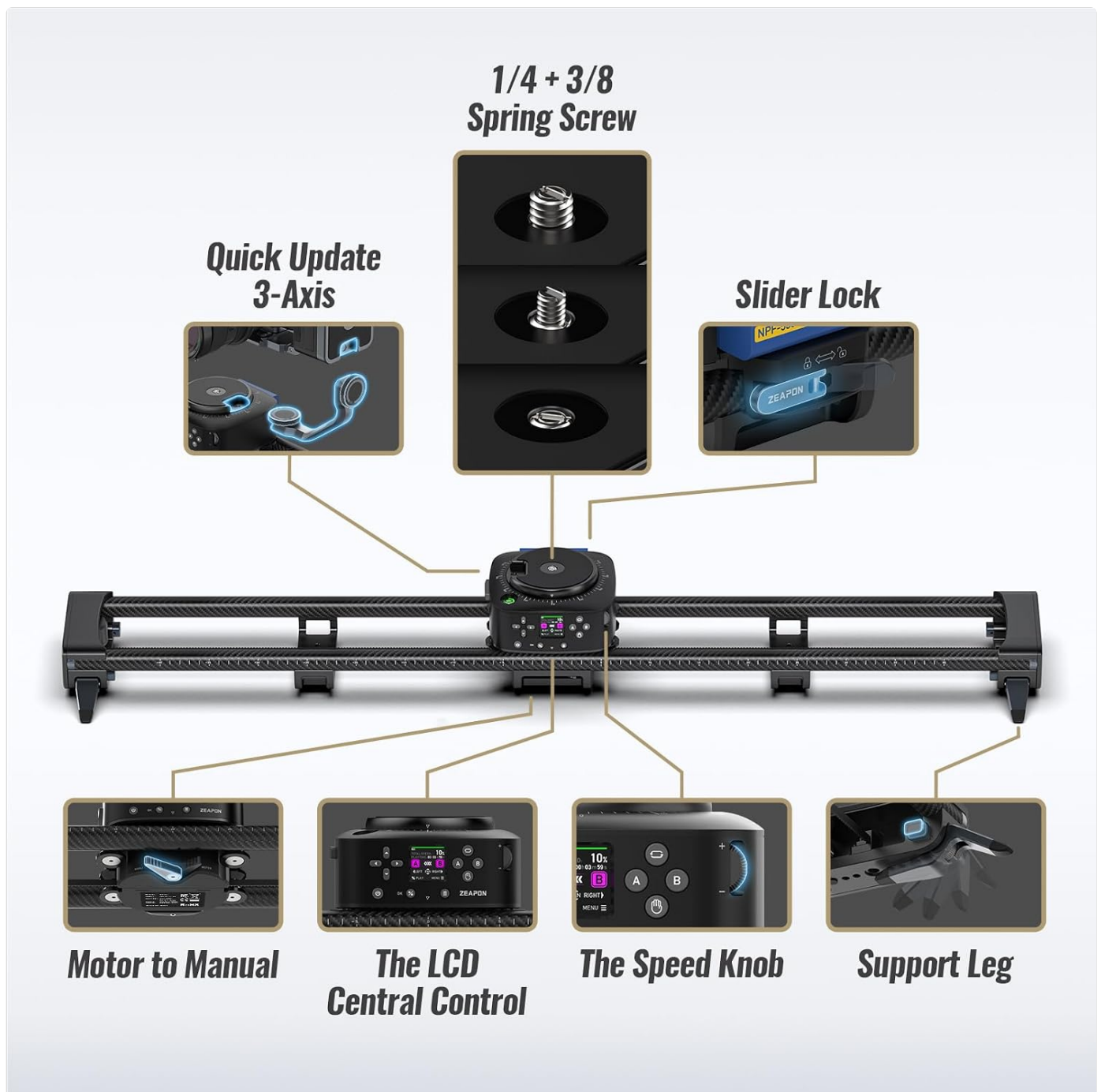
Figure 1: Overview of the Zeapon AXIS 120 Pro Motorized Camera Slider with key components labeled, including the 1/4 + 3/8 spring screw, quick update 3-axis interface, slider lock, motor to manual switch, LCD central control, speed knob, and support legs.
