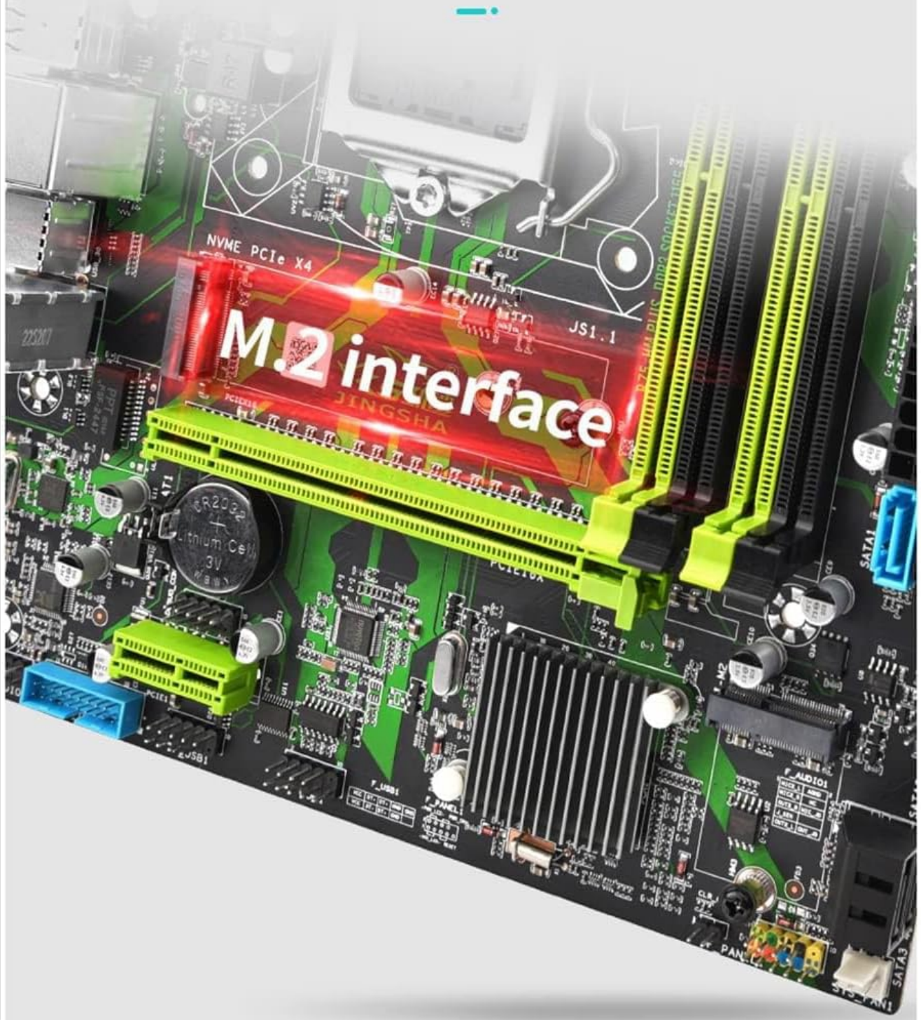
Figure 3: NVMe M.2 Interface. This close-up highlights the M.2 slot for high-speed storage devices.
