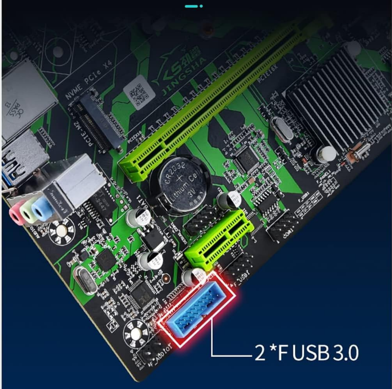
Figure 4: Front USB 3.0 Header. This image shows the internal header for connecting front panel USB 3.0 ports.
