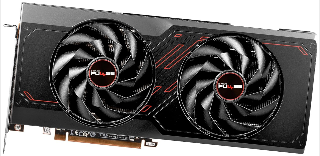
Figure 2.1: Front view of the Sapphire Pulse AMD Radeon RX 7800 XT graphics card, showing the dual fan design.
