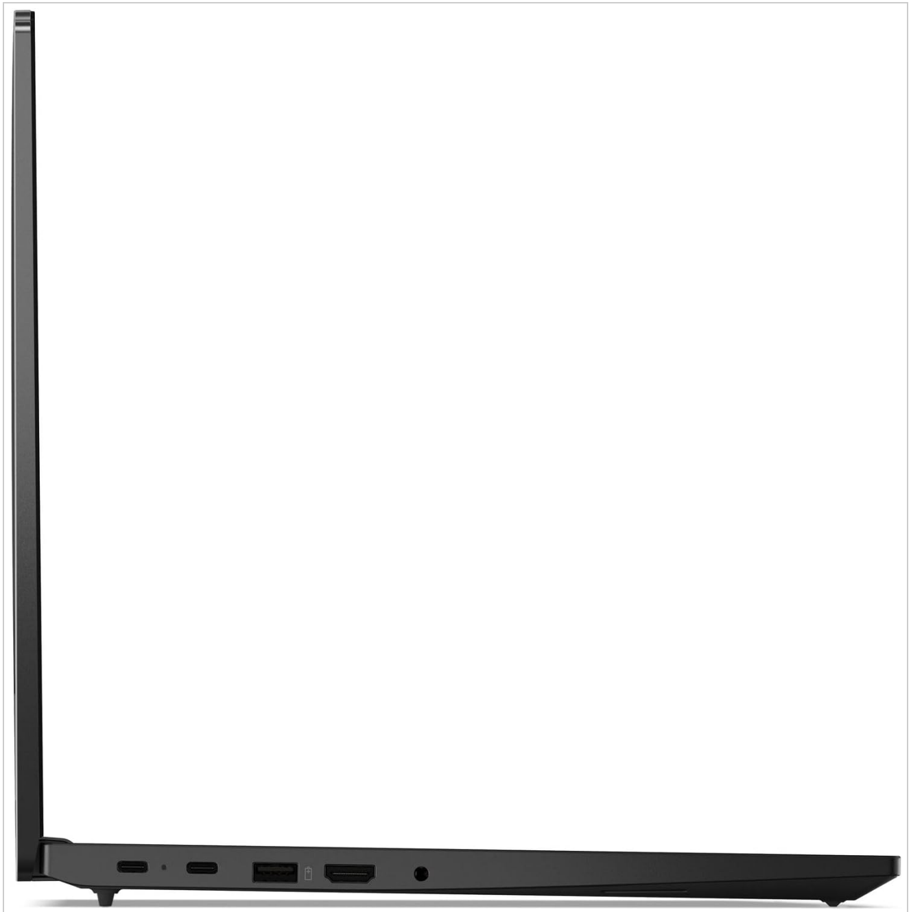
Image 3.2: Left side of the laptop showing USB-C, HDMI, and USB-A ports.
