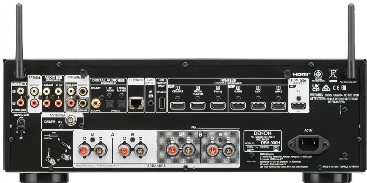
Image 4.1: Detailed view of the DRA-900H rear panel, highlighting connection points for speakers, HDMI, network, and analog audio.
