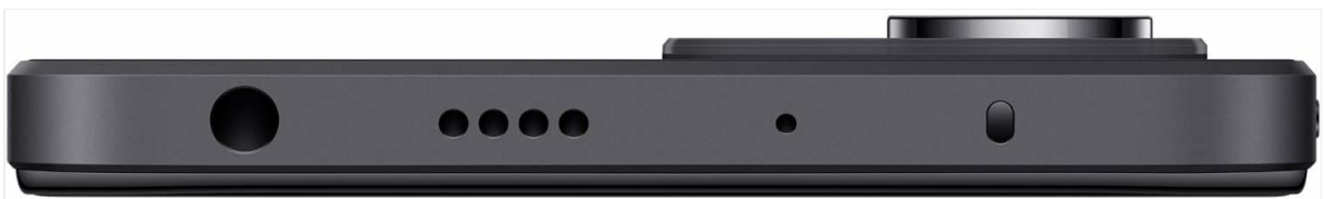
Figure 3: Top View. This image illustrates the top edge of the device, showing the 3.5mm headphone jack and a speaker grille.
