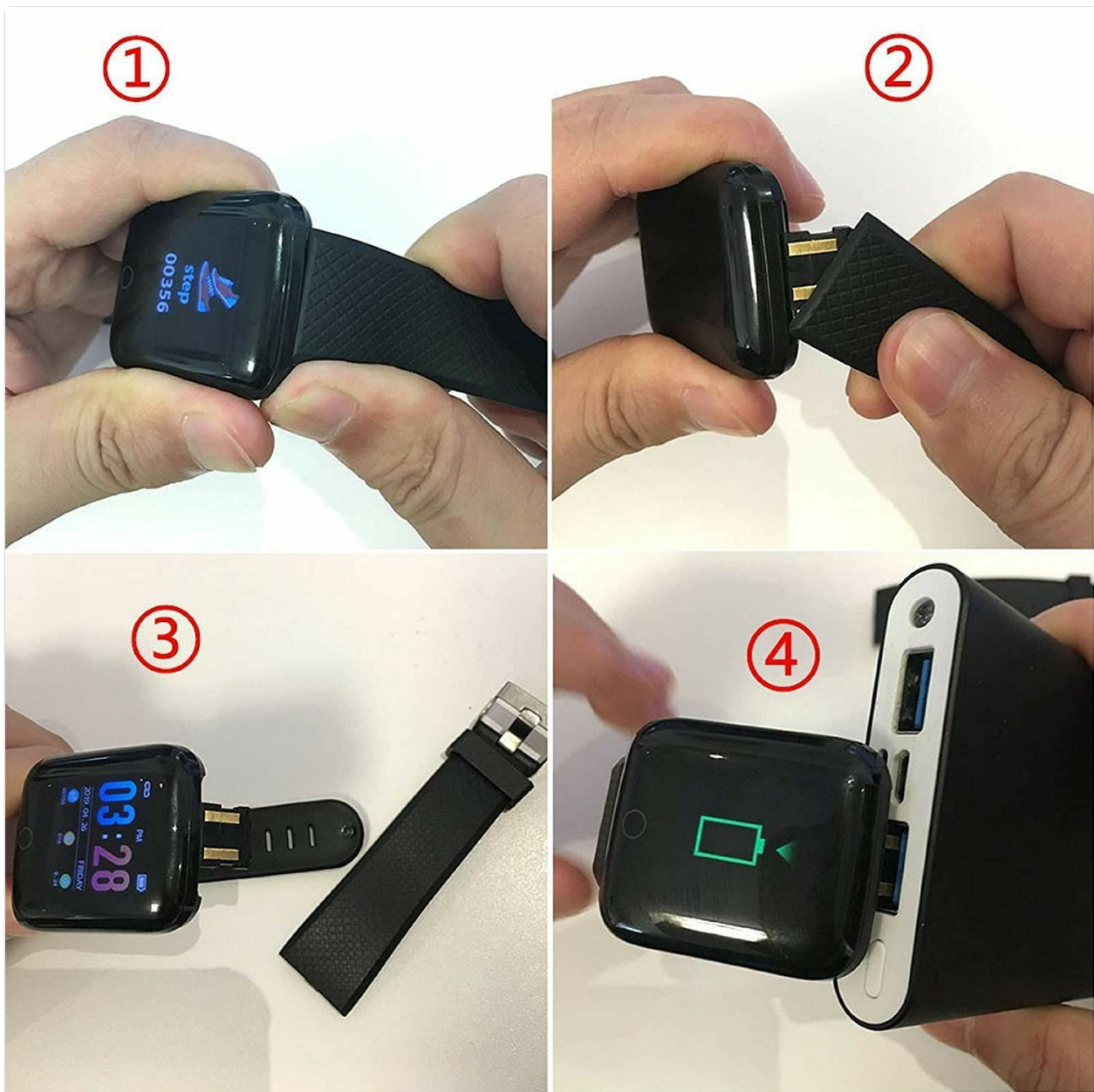
Figure 2: This sequence illustrates the simple process of charging the smartwatch: detach one side of the strap to expose the integrated USB connector, then plug it directly into any standard USB port for charging.
