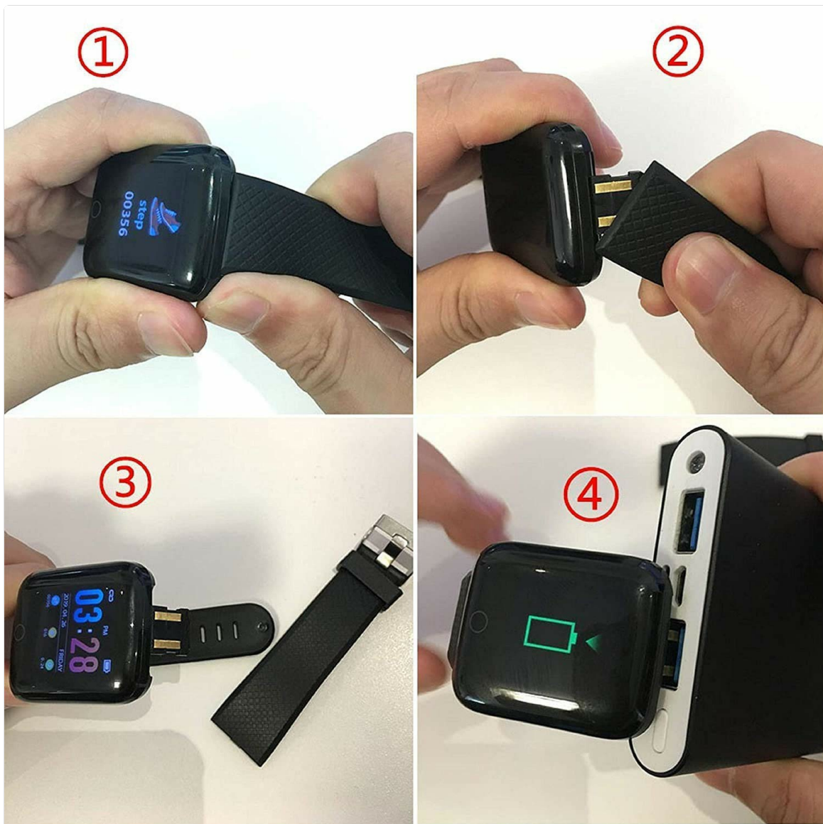
Image: A four-panel illustration demonstrating how to detach the strap and plug the watch into a USB port for charging.
