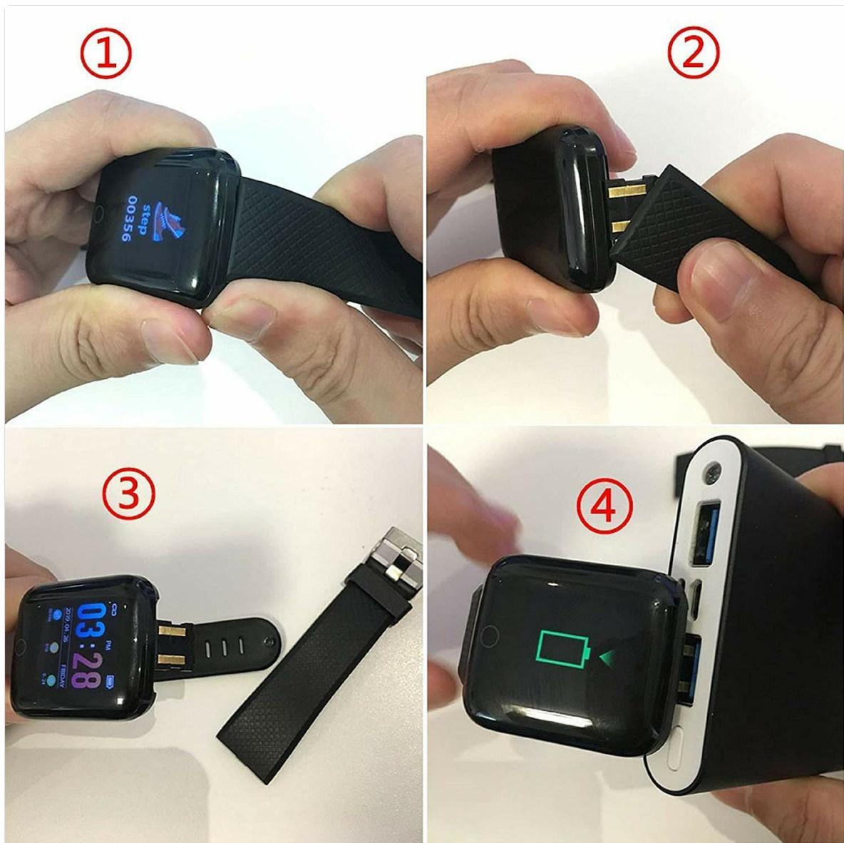
Image: Step-by-step guide illustrating how to remove the strap to access the USB charging port and connect it to a power source.
