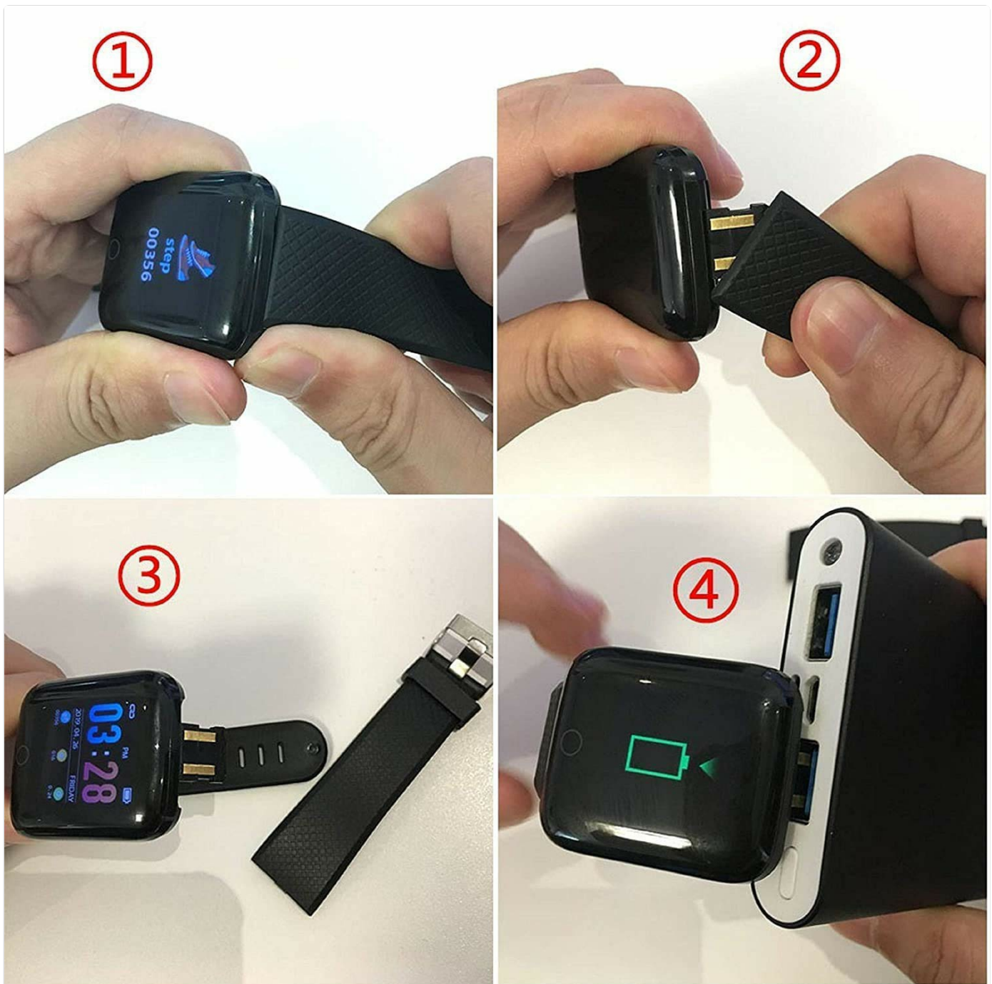
Image: Step-by-step guide for charging the smartwatch. This shows detaching the strap, revealing the USB port, and plugging it into a power source.
