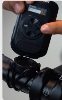
5. Fix the bike computer on the base
