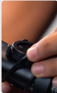
2. Place the stacked base on the bike handlebar
