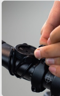
3. Cross the two rubber bands to bind the base
