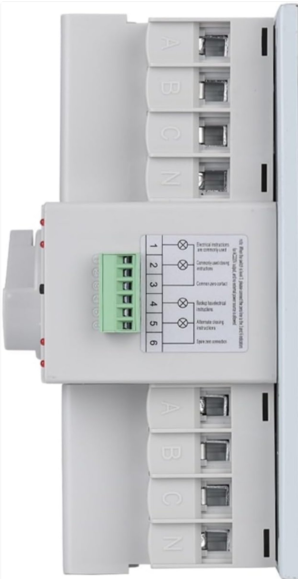
Figure 4.2: Side view of the 4-pole (4P) model, showing the terminal block for control wiring and main power connections. The label provides electrical instructions for common and backup power sources, including neutral connections.
