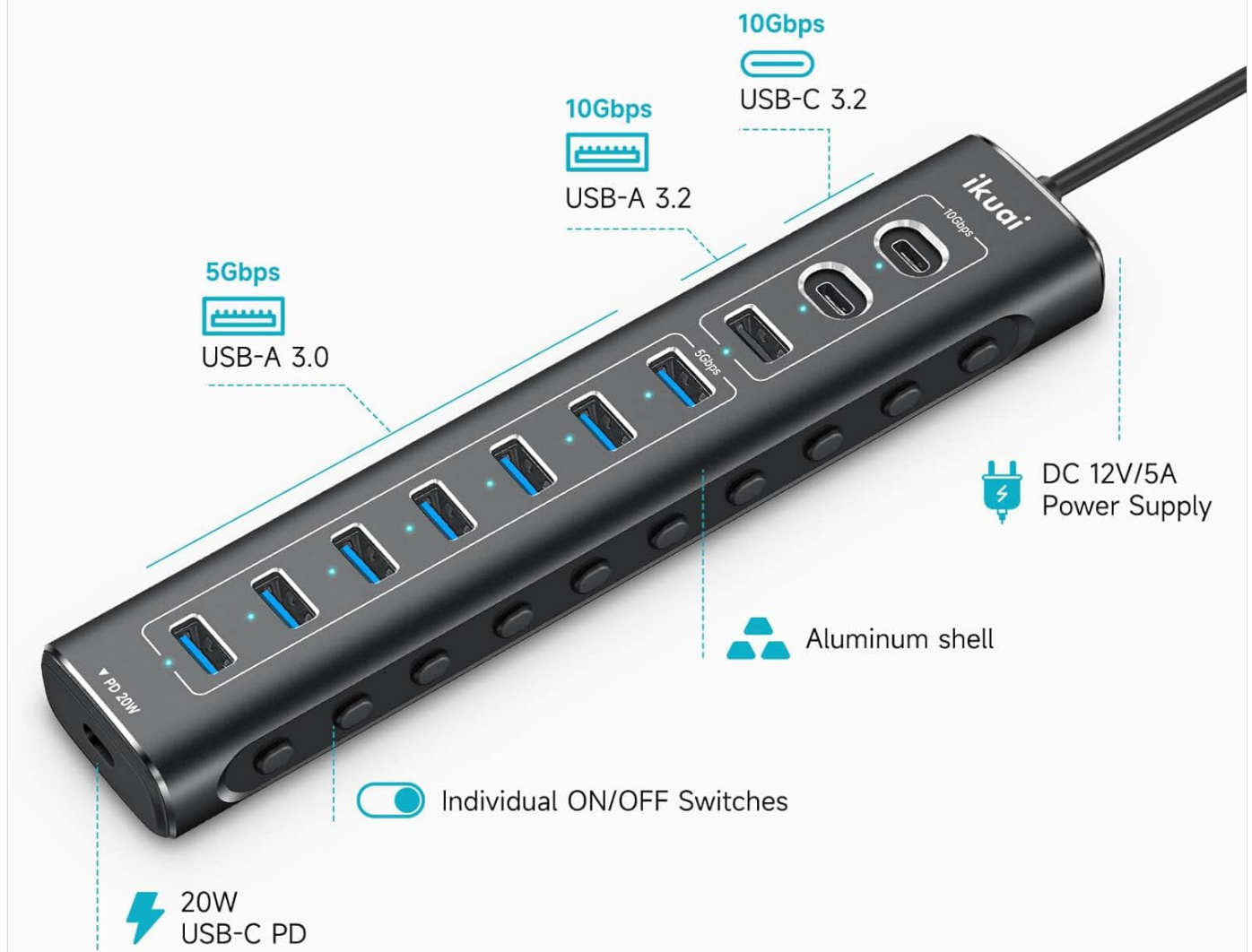
Figure 2.2: Detailed view of the 11-Port Hybrid USB Hub's various ports and their specifications.
