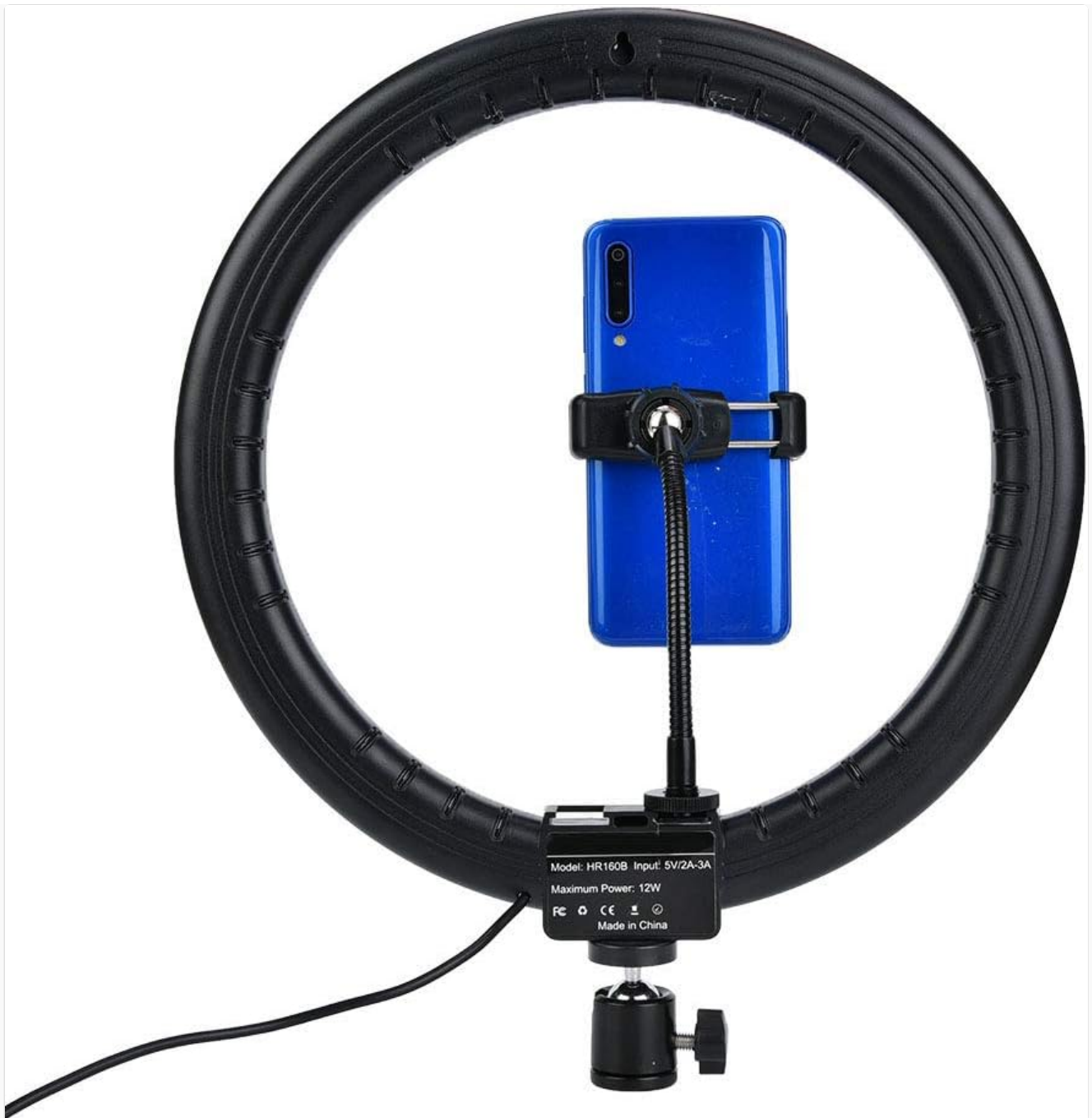
Figure 3.1: Assembled ring light with phone clip.
