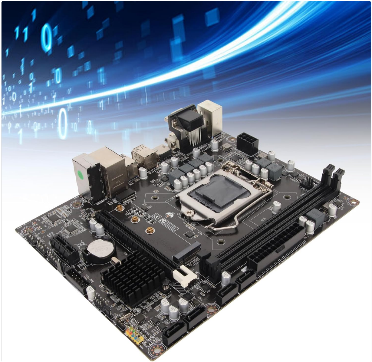
Figure 3.2: Component diagram highlighting the CPU socket, DDR4 memory slots, H310 chipset, and SATA 3.0 (6Gb/s) ports.
