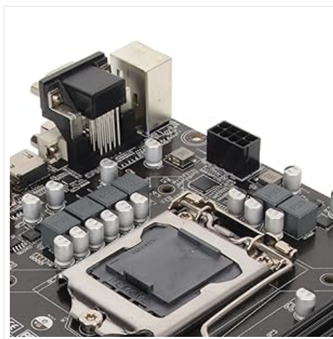
Figure 3: Close-up view of the LGA 1151 CPU socket on the motherboard, ready for CPU installation.
