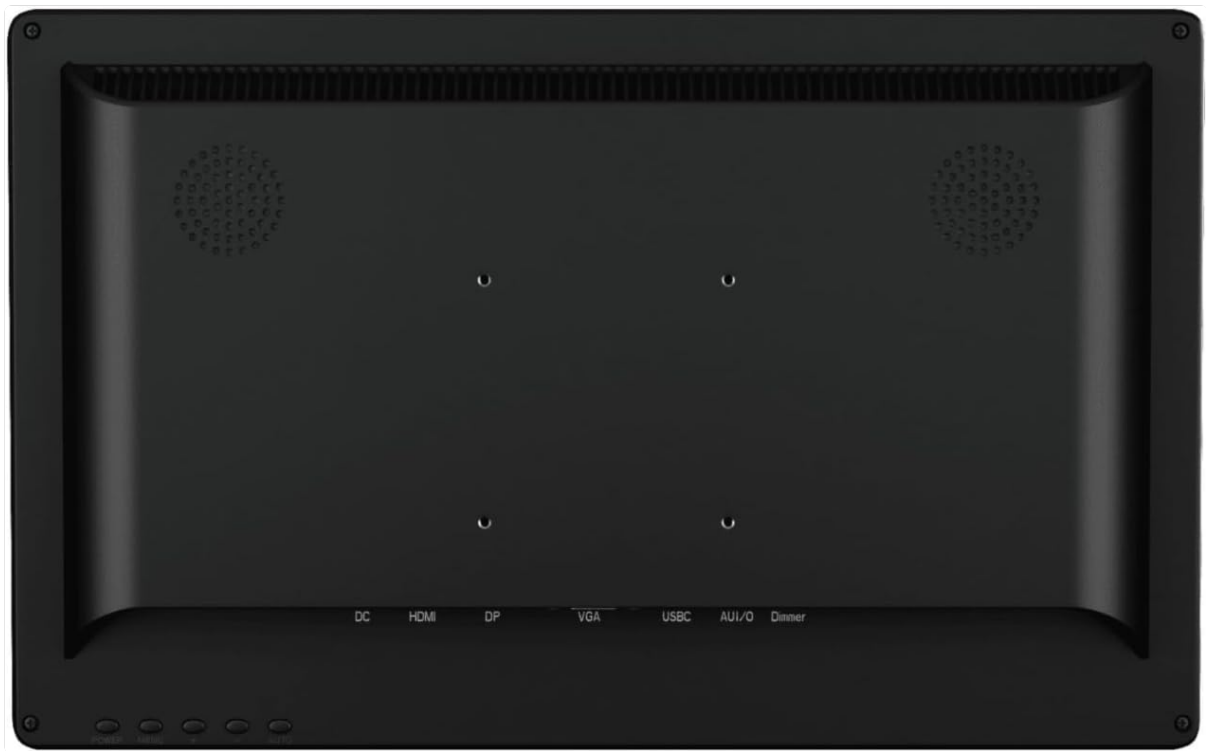
Image: Rear view of the Beetronics 15TS7 monitor, highlighting the VESA mounting holes and the various input ports.
