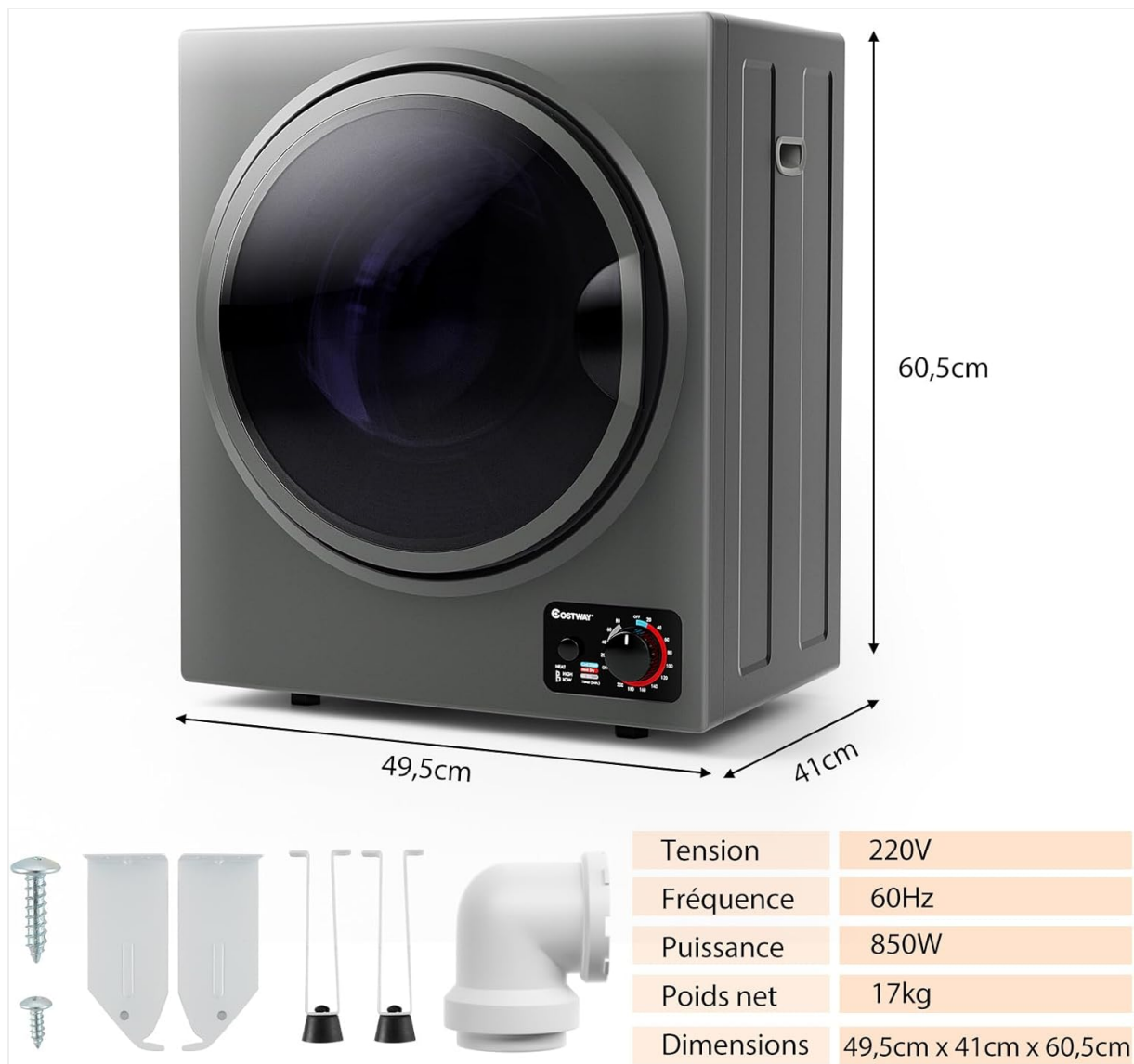
Figure 3: Dryer dimensions and included installation accessories (hanging brackets, plastic spacers, exhaust connector).
