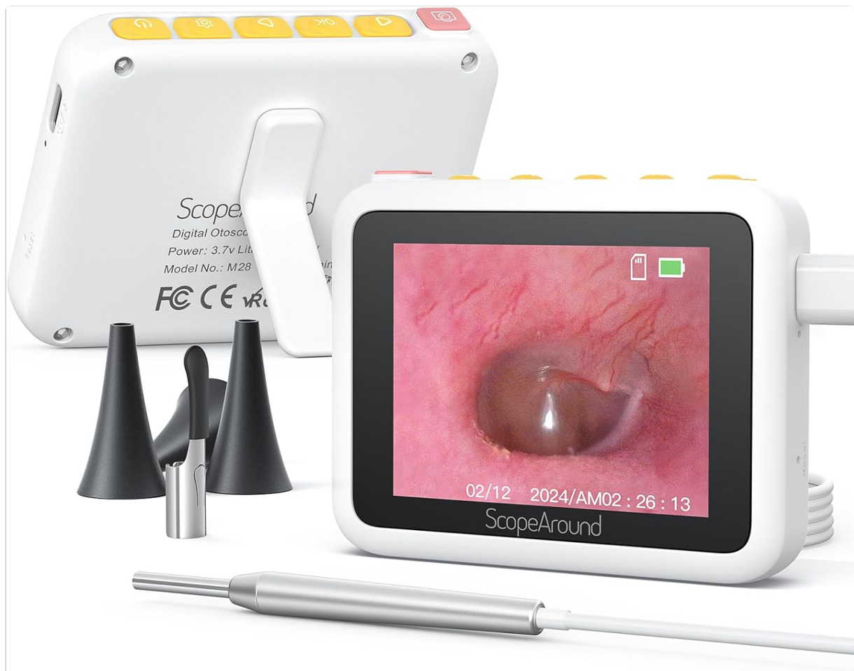
Figure 4.1: The ScopeAround M28 Digital Otoscope, showcasing the main display unit, the camera probe, and various attachments. The device is designed for ease of use and direct visual feedback.
