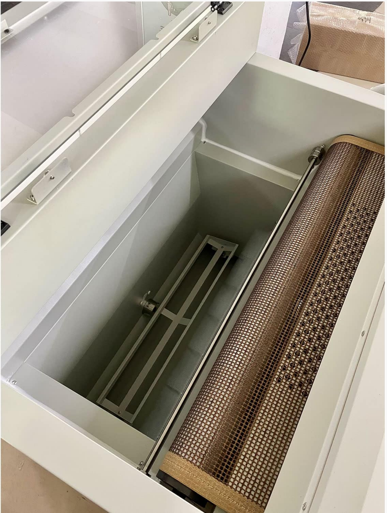
Figure 5.3: View of the powder collection and distribution system within the shaker unit.
