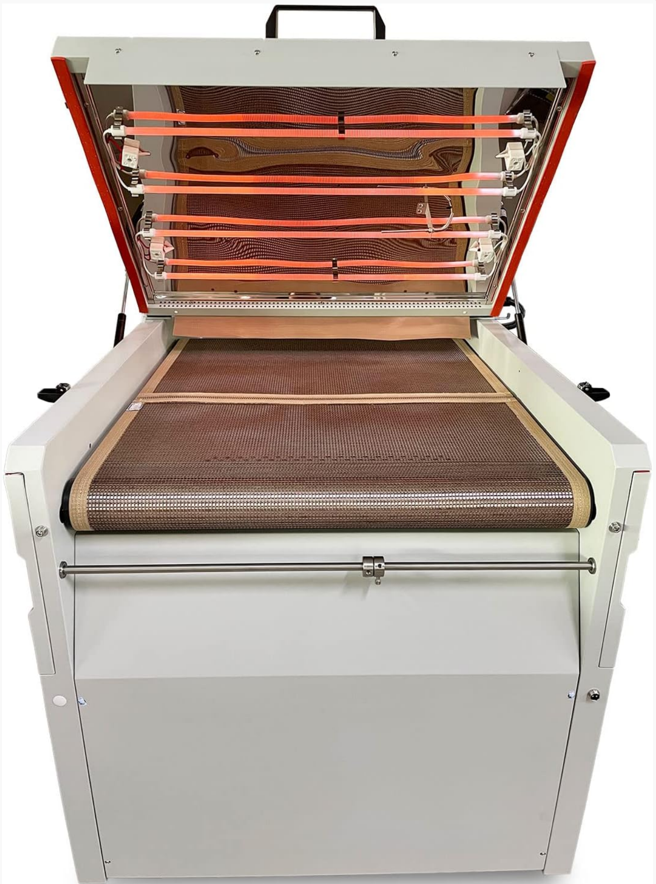
Figure 5.2: Internal view of the drying tunnel, illustrating the infrared heating elements and the conveyor belt system.
