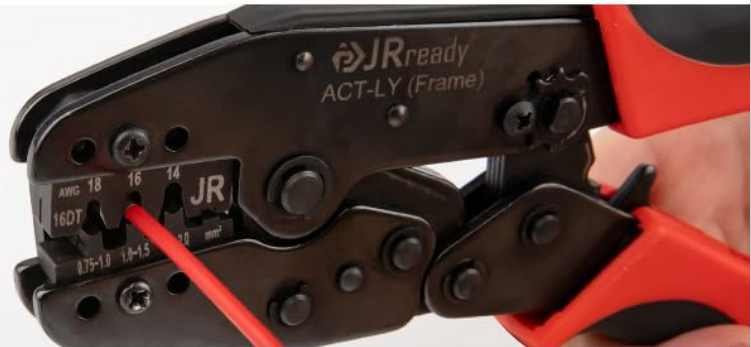
Step 2: Choose the correct positioning hole and insert the terminal.
