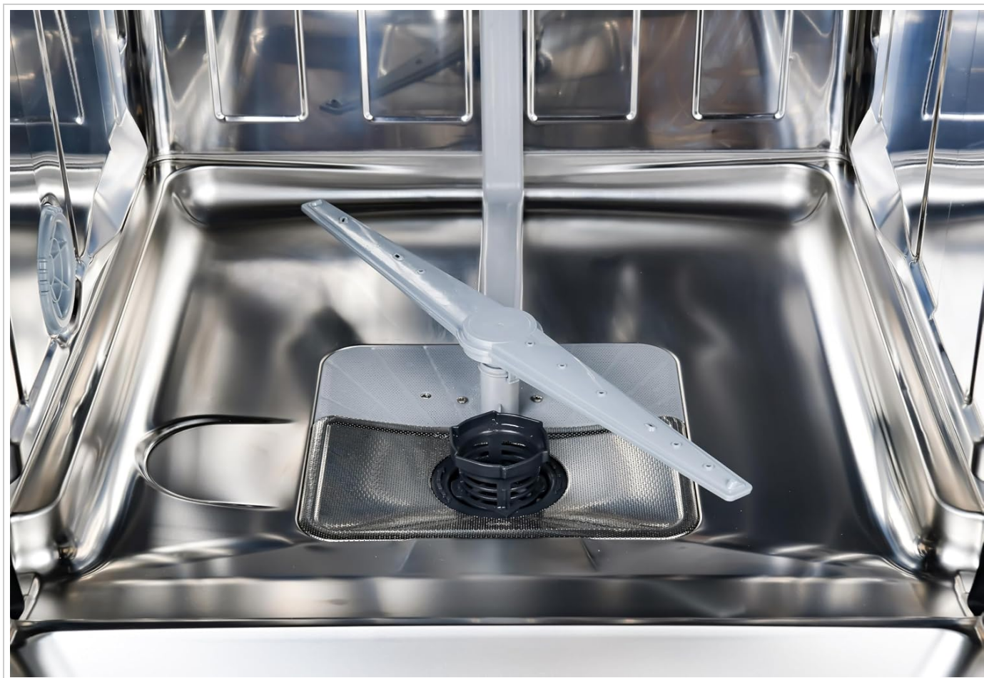
Figure 3.4: Lower Spray Arm and Filter System. The lower spray arm rotates to distribute water, while the filter system captures food particles, ensuring clean water throughout the wash cycle.
