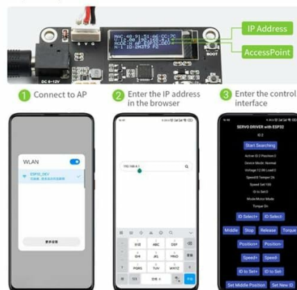
Figure 6.2: Step-by-step guide for calibrating the servo's middle position using a mobile interface. This image illustrates the process from connecting to the hotspot to setting and verifying the middle position.
