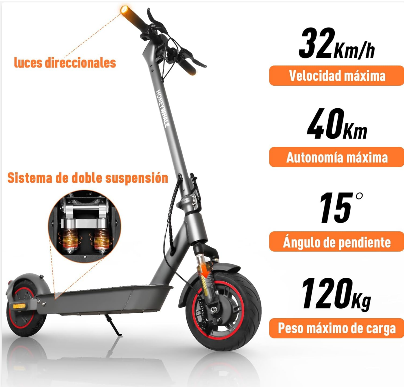
Image: Key performance specifications of the HONEYWHALE E9 MAXS electric scooter, including maximum speed, range, climbing angle, and load capacity.
