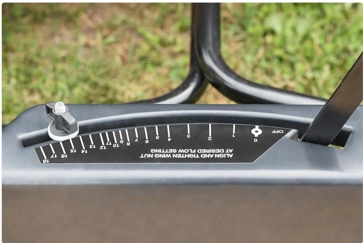
Figure 6: Detailed view of the flow setting dial on the spreader.
