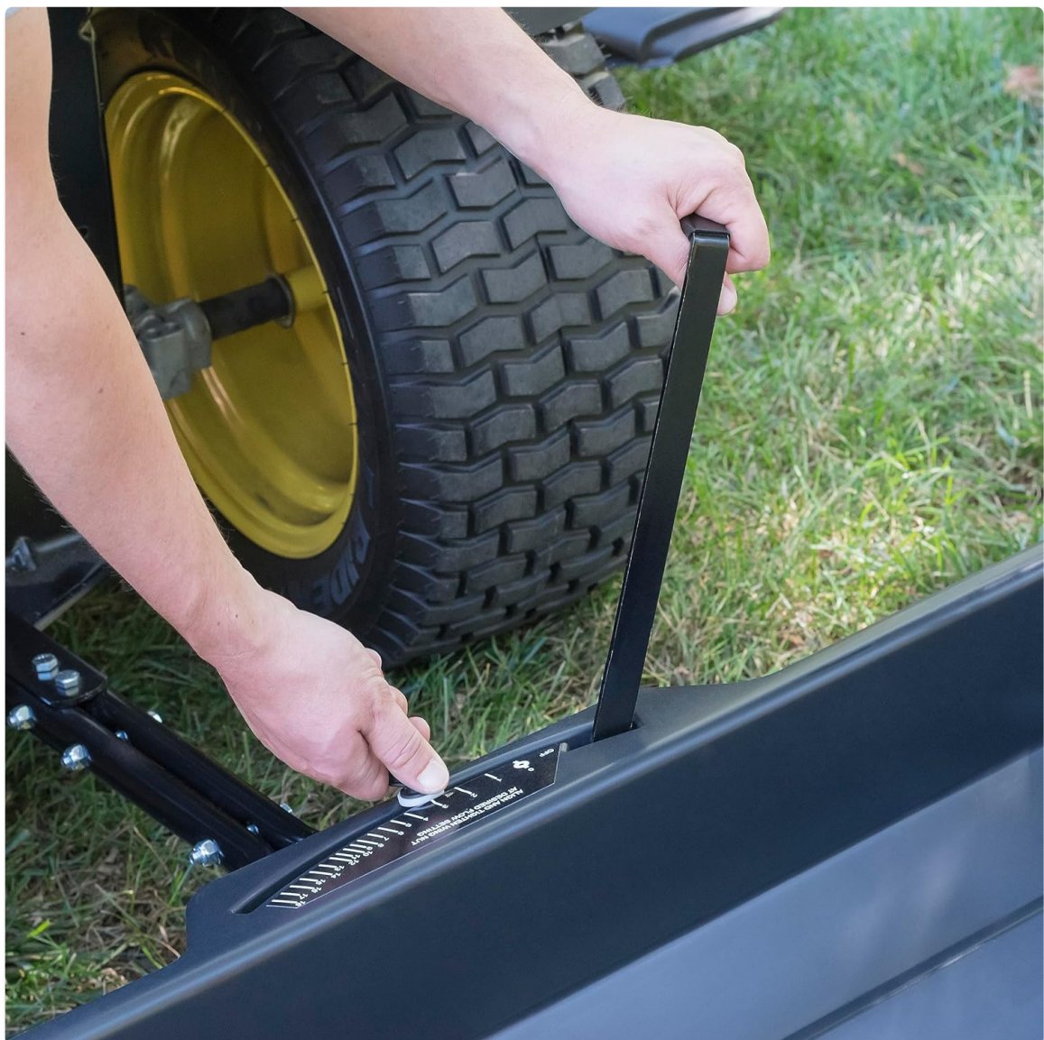
Figure 7: A user adjusting the flow setting lever for precise material distribution.
