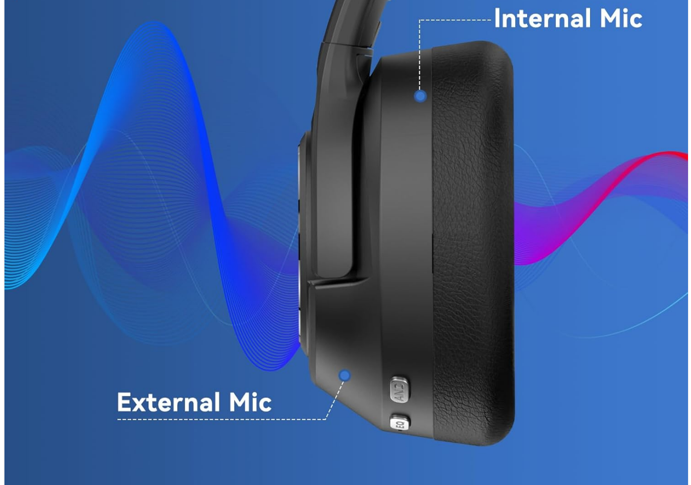
Image: Illustration of the internal and external microphones for Hybrid Active Noise Cancellation.
