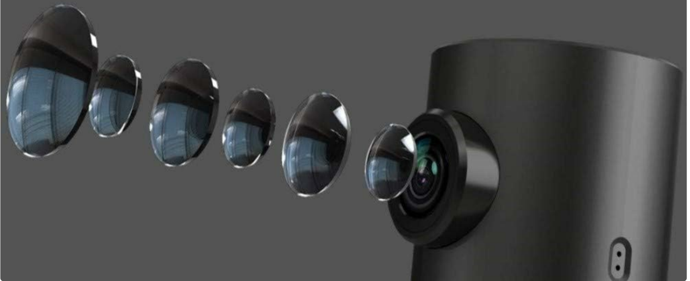
Figure 3: Details of the upgraded optical system, highlighting the 2MP CMOS sensor, 140° wide angle lens, and F2.0 large aperture for enhanced image quality.
