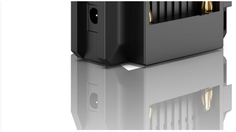
Figure 3.4: Side view of the JM300PRO unit, highlighting the DC 9-16V power input, USB-C port, and power button.
