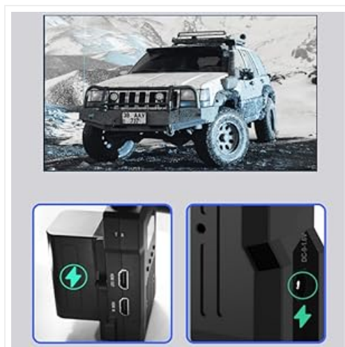
Figure 4.1: The JM300PRO offers flexible power options including NP-F batteries, DC input, and USB-C.
