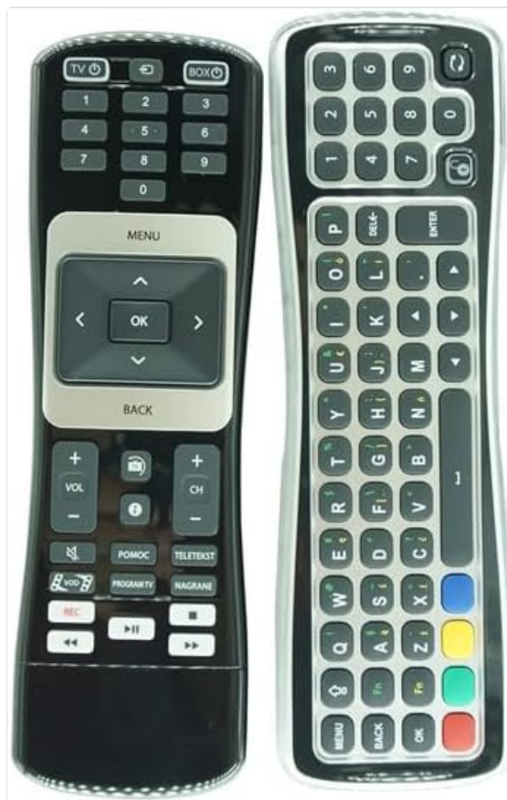
Image 1: Front (left) and back (right) view of the replacement remote control. The front features standard TV and Mediabox controls, while the back includes a full QWERTY keyboard.
