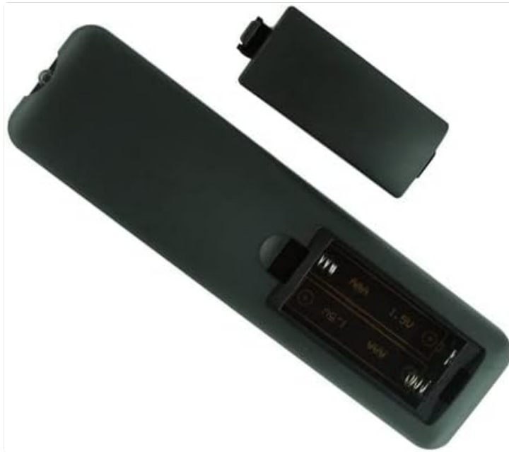
Image: Rear view of the remote control with the battery cover removed, illustrating the correct orientation for inserting two AAA batteries.
