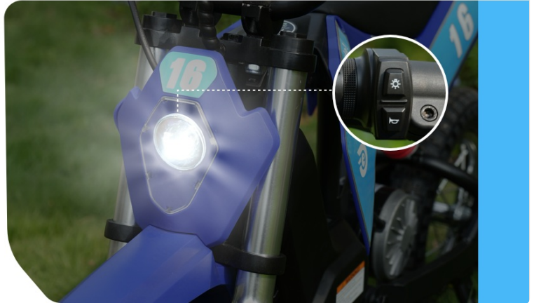
Figure 3.4: The powerful 190LUX LED headlight for enhanced visibility.
