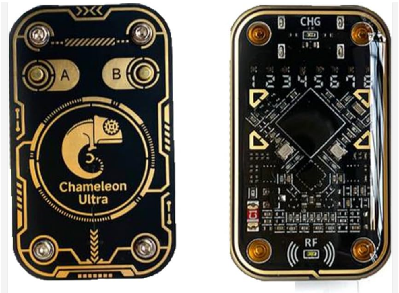
Figure 1: Front and back view of the Chameleon Ultra device, showcasing its compact design and internal components.
