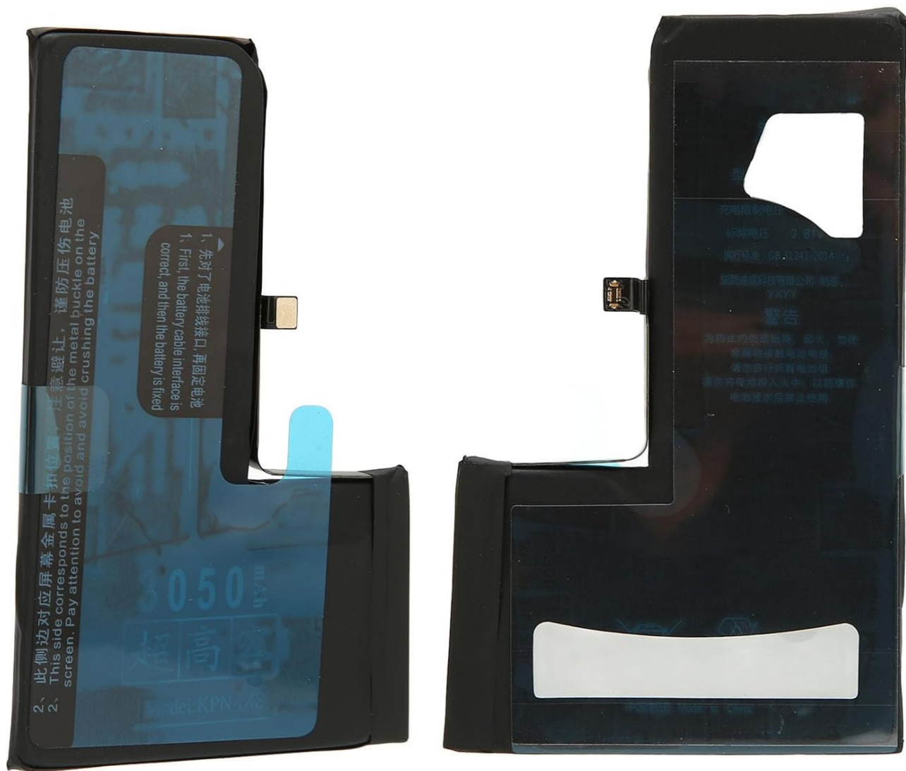
Front and back views of the graphene phone battery, highlighting its compact design and the protective film on the front.
