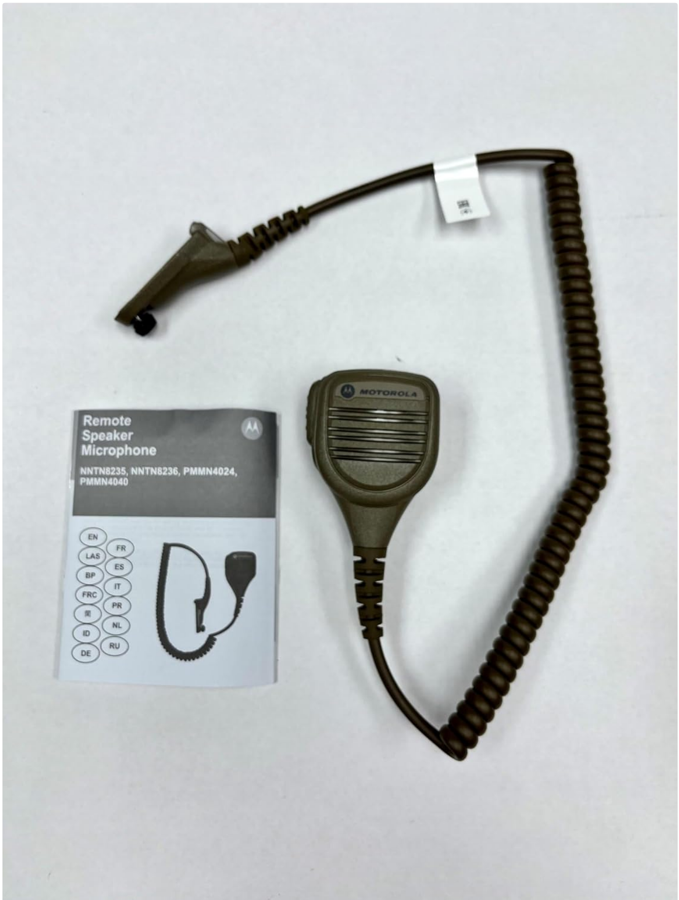
Image: Detailed view of the NNTN8235A RSM, highlighting the speaker grille and PTT button area.
