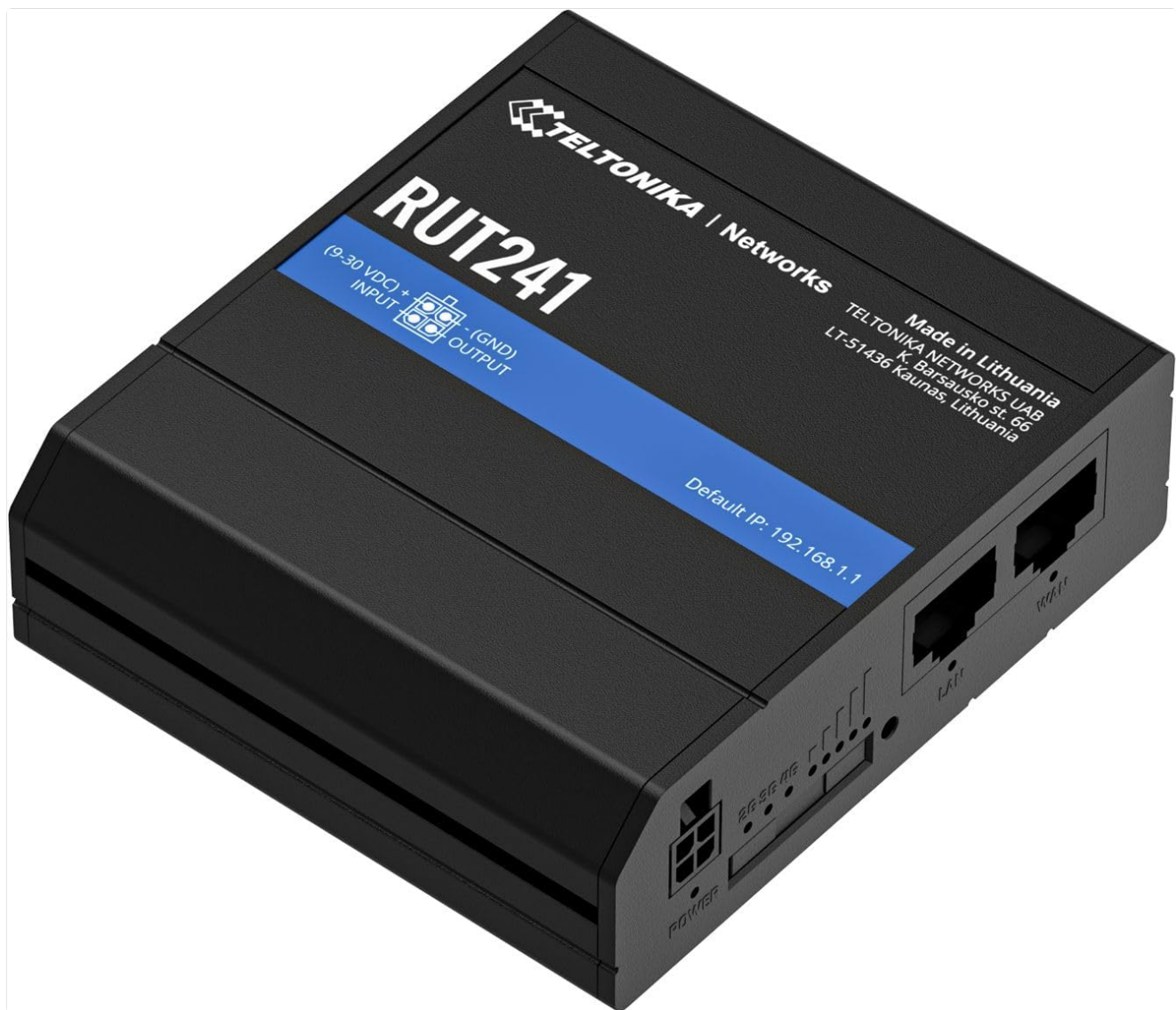
Figure 4.2: Angled view of the RUT241, highlighting the WAN and LAN Ethernet ports, the 4-pin industrial DC power socket, and LED indicators for signal strength and network status.
