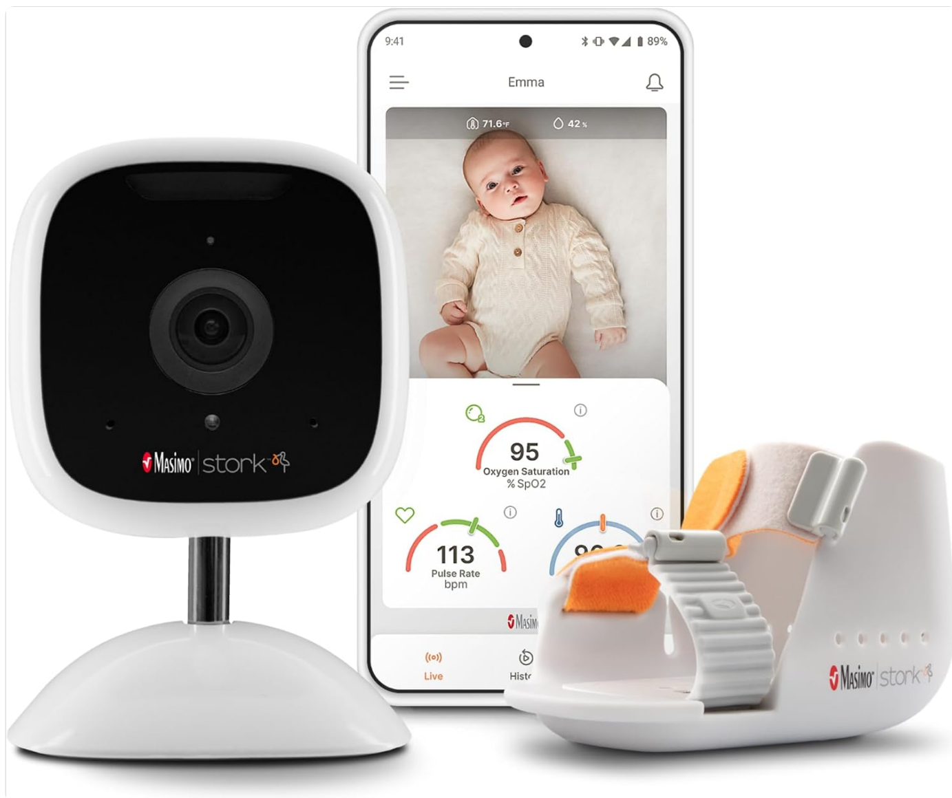
Image: The Masimo Stork Vitals+ system, showcasing the camera, the sensor boot, and a smartphone displaying the monitoring app interface with vital signs.
