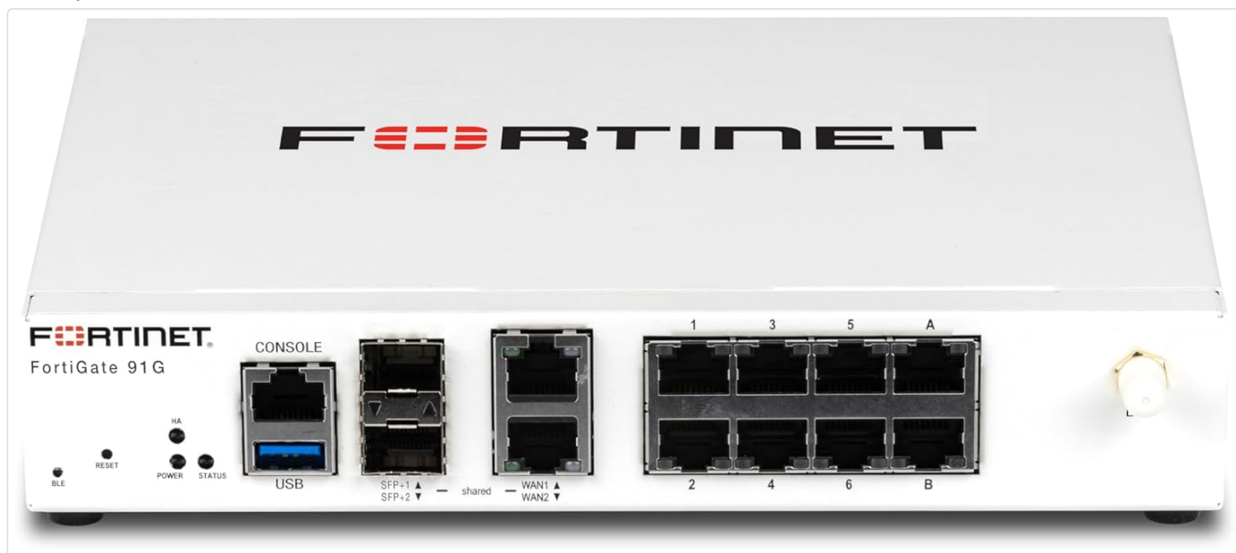
Figure 2.1: Front view of the FortiGate 91G appliance, showing all ports and indicators.
