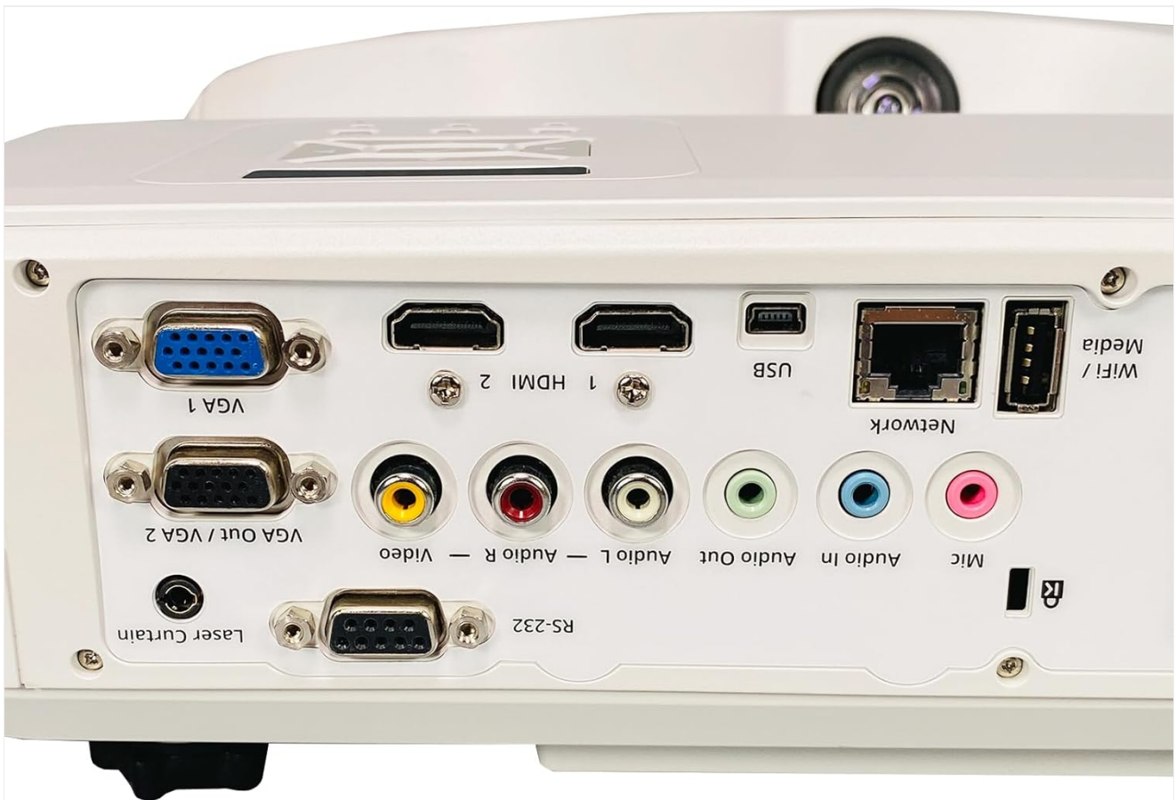
Figure 4.4: Detailed close-up of the Nureva NPSi-1 projector's rear connectivity panel, showing individual ports such as VGA 1, HDMI 1, HDMI 2, USB, Network (RJ45), Audio In/Out, Composite Video, and RS-232.
