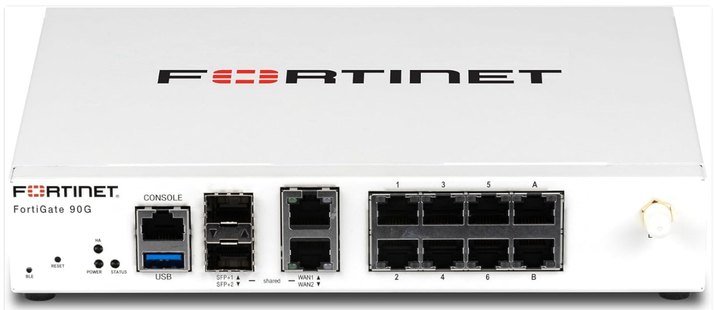
Figure 2.1: Front view of the FortiGate 90G appliance, showing the console port, USB port, SFP+ ports, WAN ports, and GE RJ45 ports.
