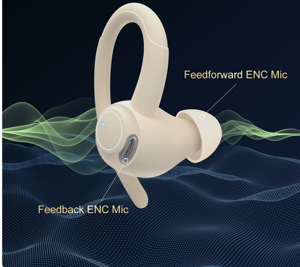
Image 3.2: A detailed view of the Jesebang YT18 earbud, pointing out the locations of the feedforward and feedback ENC microphones for effective noise cancellation.
