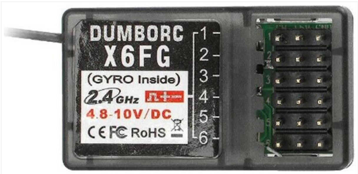
Figure 4: Close-up view of the receiver's label, indicating "P6F(G) (GYRO Inside)", 2.4GHz, and voltage range.
