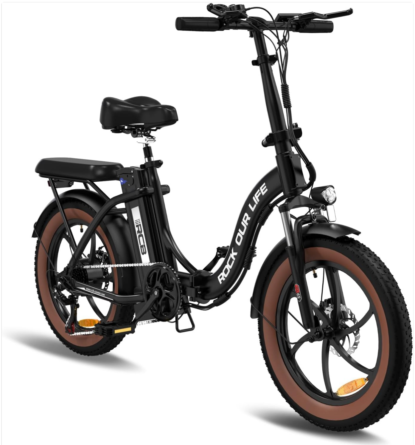
Figure 2.1: Overview of the RCB RK6 Electric Folding Bicycle.
