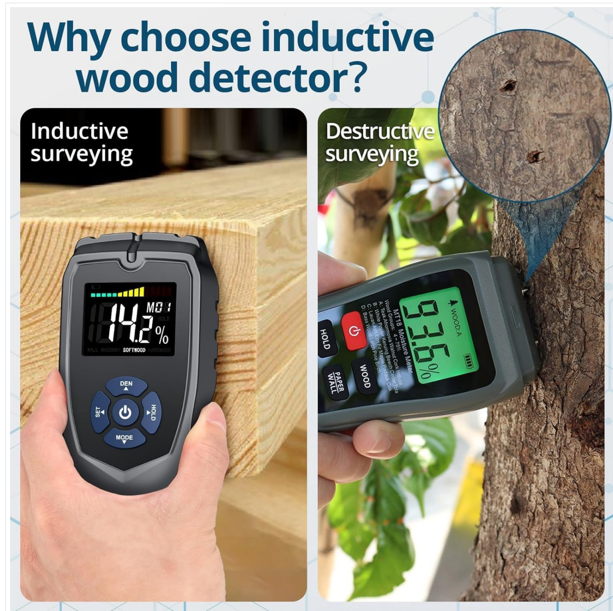
Image 7.3.1: A visual comparison between inductive (pinless) surveying, which leaves no marks, and destructive (pin-type) surveying, which creates small holes in the material.
