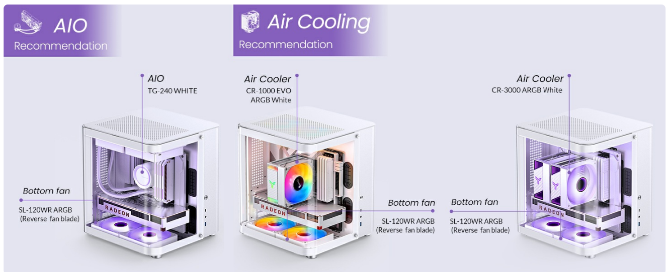
Image 2.6: Cooling Recommendations. This image provides visual examples of AIO and air cooler installations, along with recommended fan placements for the JONSBO TK-1 case.
