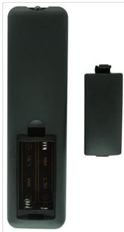
Figure 2: Back view of the remote control, illustrating the open battery compartment ready for battery insertion.
